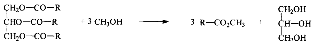
Figure 3: Transesterification of triglycerides with methanol.
